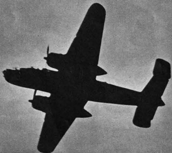
Wide-set fins and rudders on the B-25 are visible from nearly every angle. On B-25H and J (see June Journal) dorsal turret has been moved forward to straddle leading edge of wing. Below, a B-25 leaves the deck of the carrier Hornet on its way to bomb Tokyo.
